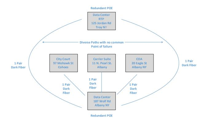
Fiber between the Data Centers (RTP and Wolf Rd) must take diverse paths and have no common point of failure. In addition, dual building POEs are mandatory for the Data Centers to ensure no contractor work can impact both paths at the same time.
